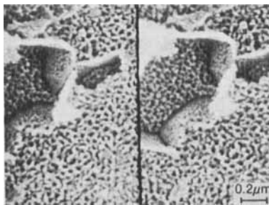
FIGURE 3 CAA oxide after heating in air at 330°C for 1200 hours. Some thickening of the cell walls has occurred.
